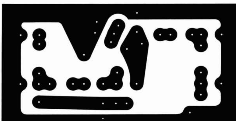
fig. 2. Foil side of the printed-circuit layout for the wideband amplifier.
